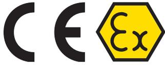
The products must be equipped with the appropriate identification plate which must have, in addition to the CE marking, the specific marking of explosive protection (**Epsilon-x**, in the hexagon) followed by the **group** (I or II) and **category**; for **group II**, the letter **G** is added for equipment for Gas while equipment for dust is identified by the letter **D** (Dust).
