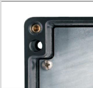
Corrosion-resistant stainless steel (complete with retaining washer) for flat blade screwdriver and PH screwdriver. The assembly holes are outside the sealed area.
